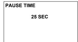
Here the operator can set the interval time between each scrape movement. By using these buttons:
