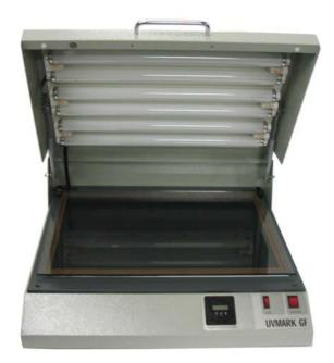
2 - lift the glass plate up to the blocking device :
